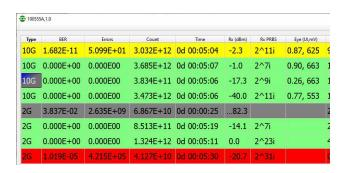
Error rate, error count, bit count, and test time are displayed for each channel in a grid format. Colors are used to indicate lock, error free operation, error history, and real-time bit errors.
